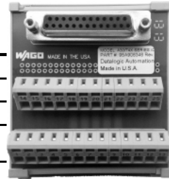
Figure 8 – A30/T4x-Series I/O Block
