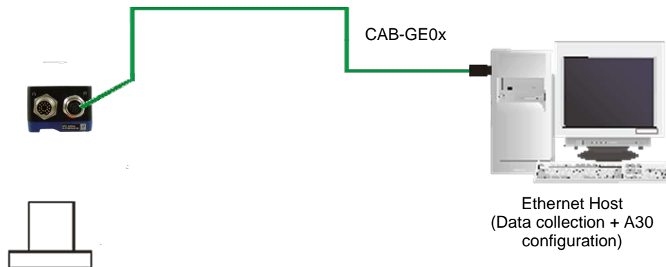
Figure 45 - Standalone Layout to Ethernet Host (Point-to-Point)
